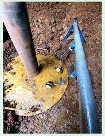
SOIL FIELD DRY DENSITY BY CORE CUTTING METHOD
